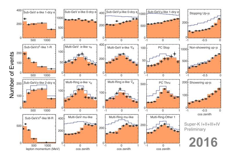
Zenith angle and momentum distributions for atmospheric neutrino subsamples used for an analyses by Super-Kamiokande to study subleading effects, preferences for mass hierarchy and  $\delta_{CP}$ , as well as searches for astrophysical sources such as dark matter annihilation.
