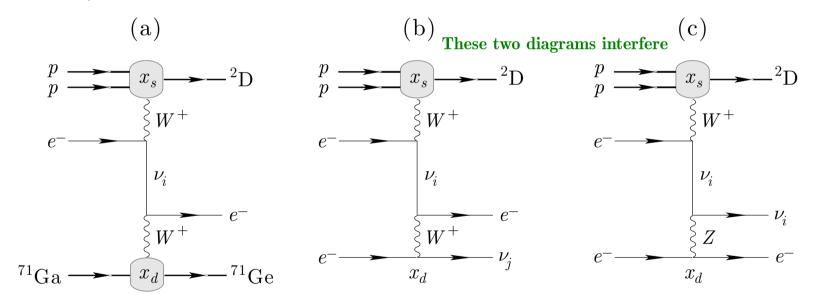
The Figure illustrates the detection of pep neutrinos with gallium (a) and electron (b,c) targets. Similar to the pp neutrino case, the diagram sets (c) and (d) interfere. While the final electron in the detector vertices of the diagrams (b,c) may have a momentum above the Cherenkov threshold, the current water-Cherenkov detectors SK and SNO+ are insensitive to the pep neutrinos.
