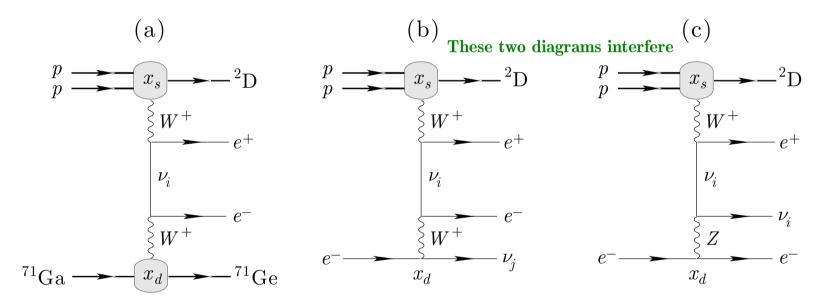
The Figure illustrates the detection of pp neutrinos with gallium (a) and electron (b,c) targets. Unfortunately, the final electron energies in the reactions (b,c) are too low to be detected by Cherenkov method.
