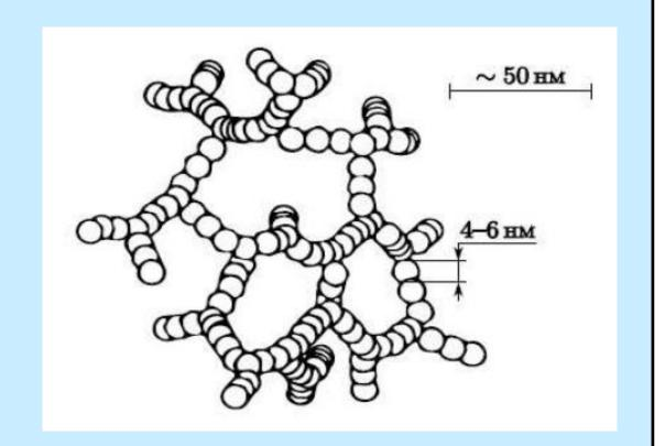
Aerogel consists of spheres of amorphous silica with a diameter of several nanometers, connected in chains (such as "caterpillars"), forming a chaotic three-dimensional structure.
