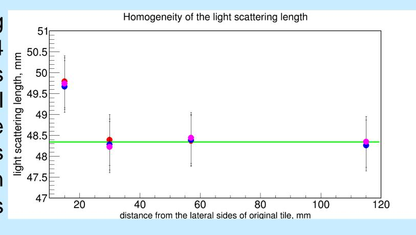
The figure shows the distribution of the light scattering length for 145 aerogel blocks. The mean of the light scattering length is 50 mm for the aerogel tile 20 and 30 mm. All aerogel blocks have the light
